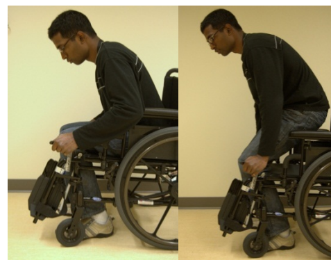
Figure 2: Photographs of subject using handle to assist with STS. Left image: subject flexing trunk; Right image: subject pushing on handle during STS.
